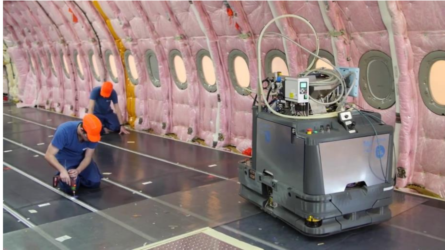
Figure 16. Mobile cobot used by Airbus Aero 26 to produce some parts of A380
