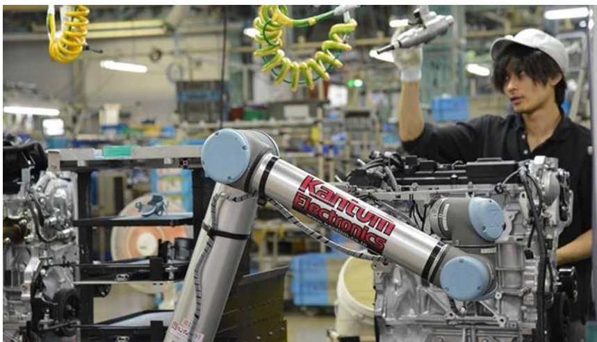
Figure 6. Picture of a collaboration between a worker and a cobot in assembly process
